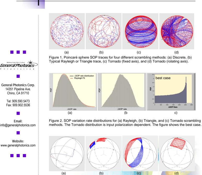
Figure 3. (a) Manual adjustment of SOP from H to V state. (b-d) SOP patterns generated in polarization modulation mode using different combinations of waveforms on different channels of the polarization controller.
